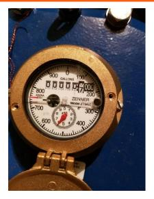
Water meters at Well #2 and Well #3 track how much water our system pumps on a monthly basis. In summer months, this amount can be as high 8,500,000 gallons in a month.
